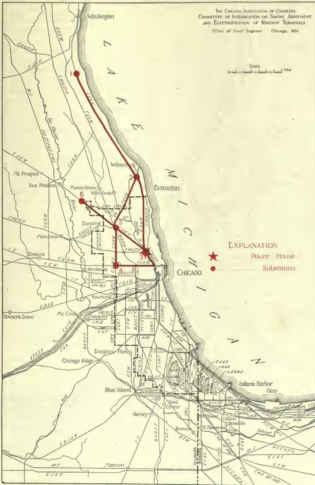
FIG. 685. LOCATIONS OF POWER STATION AND SUBSTATIONS FOR THE 2,400-VOLT D. C. SYSTEM. CHICAGO & NORTH WESTERN RAILWAY
